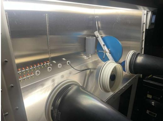
Gloveport cover used for leak checking and is not included
