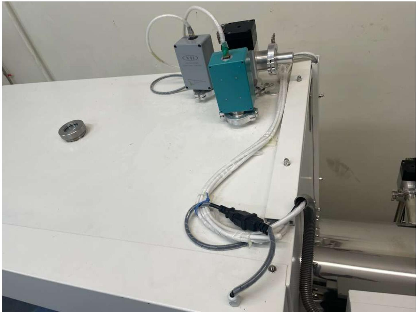
View of the O<sub>2</sub> & H<sub>2</sub>O sensors, purge valve & quartz window located on top of the glovebox.
