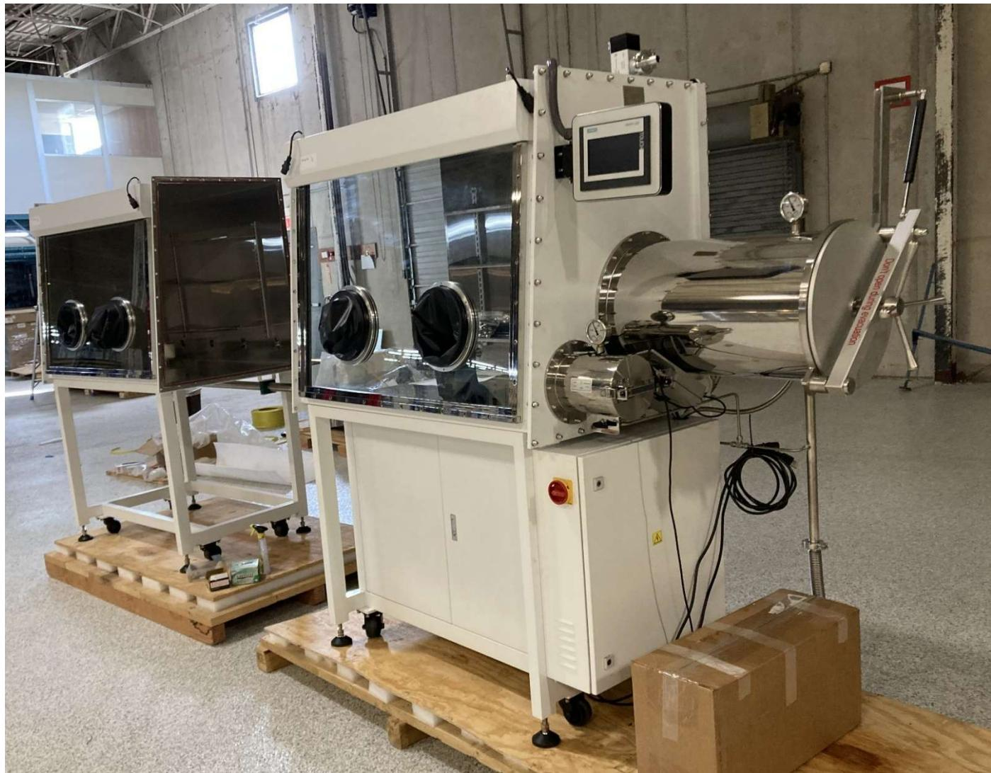
**The 2 halves of the system are easy to join, bolt and seal the attached gasket**
