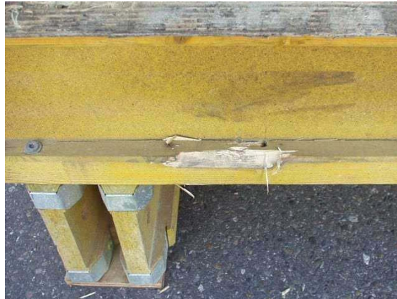
Photo 12: Permissible chipped edges
