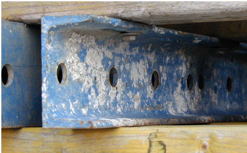
Photo 5: Permissible concrete surplus on the steel waling
