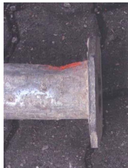
Photo 9: Impermissible large crusts of concrete and dent on outer tube
