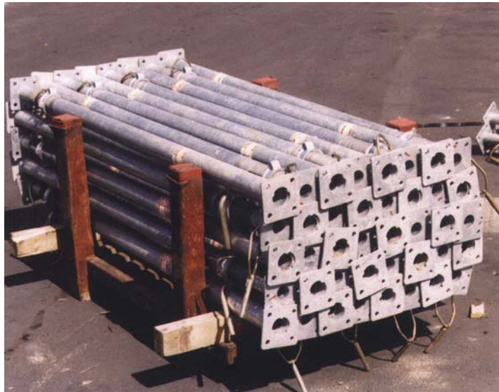
Photo 8: Used props, required cleaning condition
