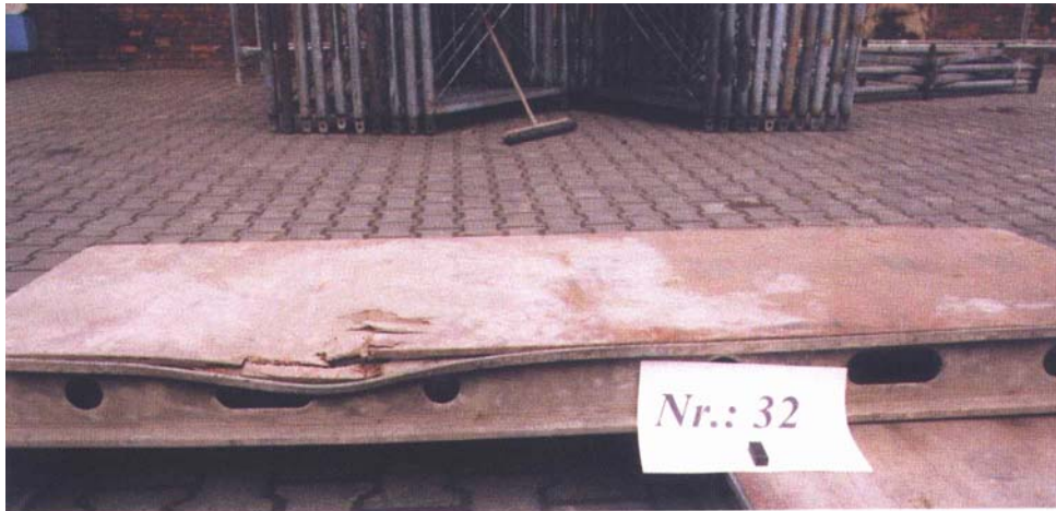
Photo 16: Non-permissible damage to the frame profile
