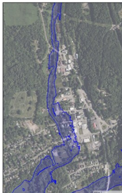
10-Year Storm Inundation Limits (No Floodwalls)
