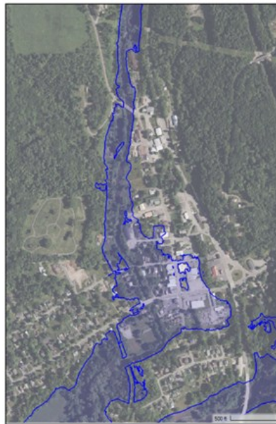
100-Year Storm Inundation Limits (No Floodwalls)
