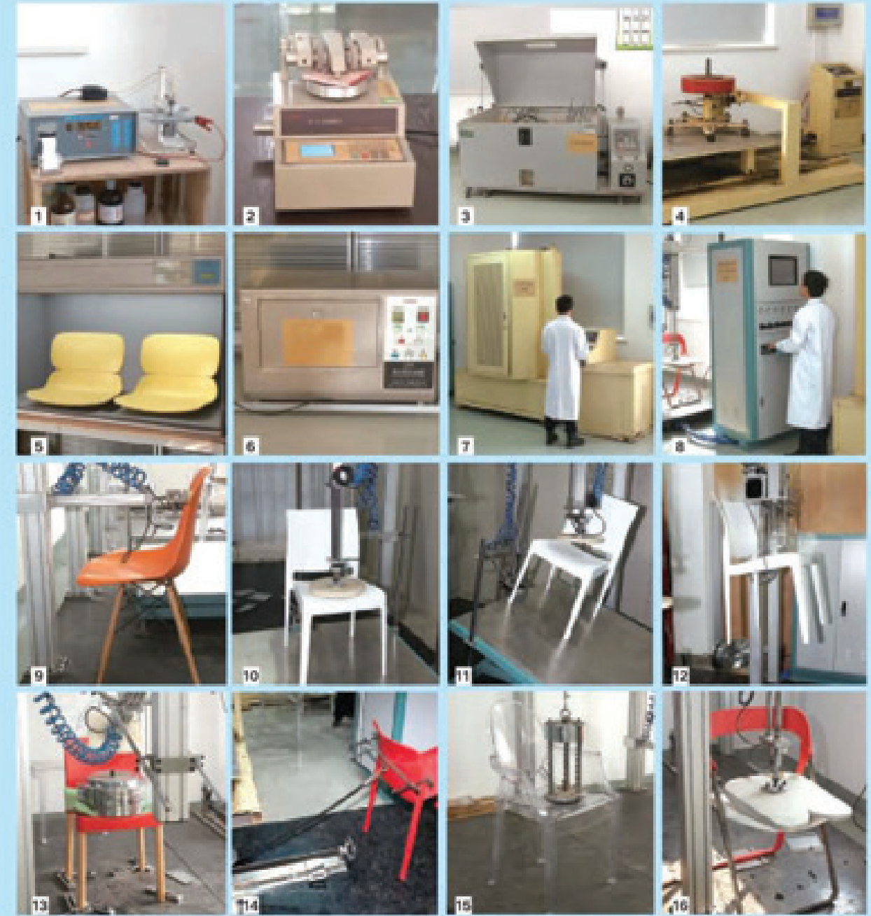
1.Salt Spray Testing Chamber 2.Castor Testing on load-bearing and stability 3.Color Assessment Cabinet 4.Ultraviolet Aging Test Chamber 5.Five Star Legs Compression Test Machine 6.Centre Control Unit Machine 7.Rearwards Overbalancing 8.Seat Static Load Test 9.Leg Sideways Static Load Test 10.Dropping Test 11.Back Static Load and Fatigue Test 12.Forwards Overbalancing 13.Seat Impact Test 14.Seat Fatigue Test
