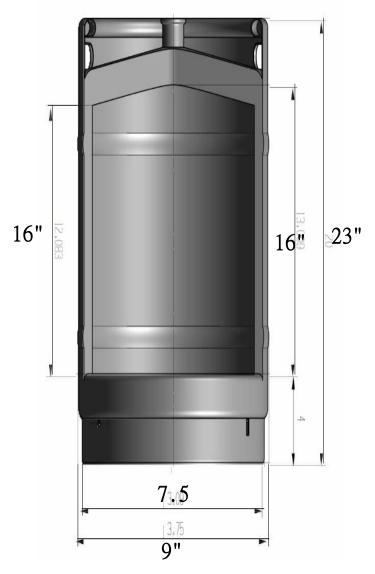
**ENGINEERING SPECIFICATION:** 304 STAINLESS STEELWITH WELDED IN INTREGAL DRAIN 1-1/2"; 3/4" FITTING FOR FLUSH VALVE; BRACKETS FOR MOUNTING; **NO SHARP EDGES. WT. 12 LBS**
