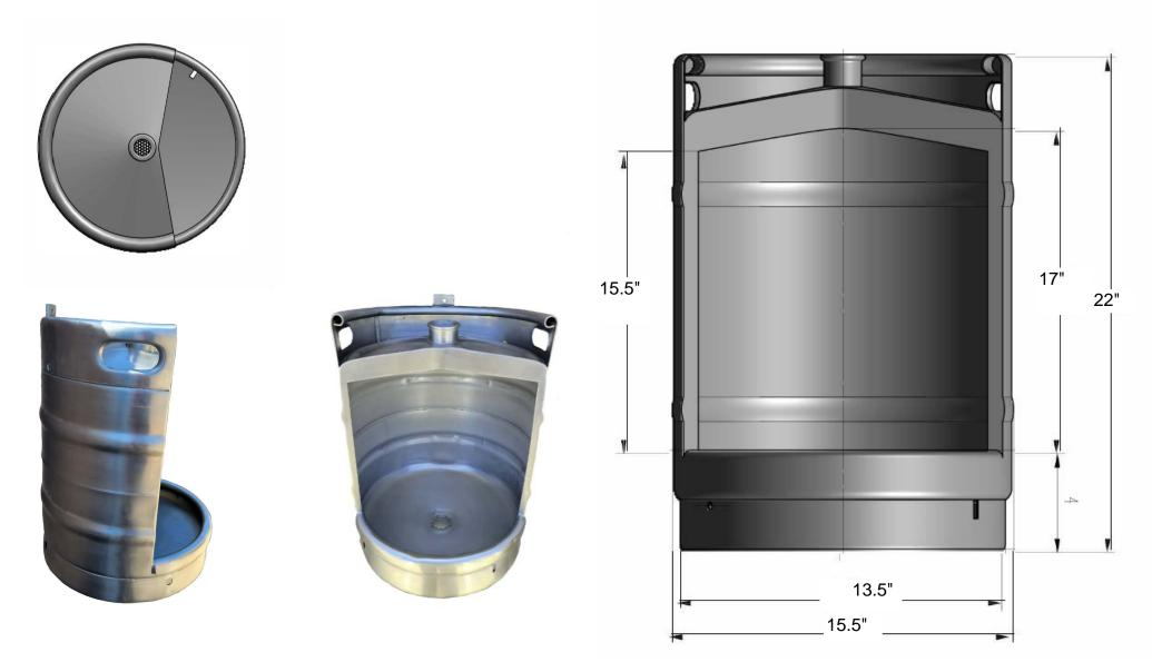
**ENGINEERING SPECIFICATION:** 304 STAINLESS STEELWITH WELDED IN INTREGAL DRAIN 1-1/2"; 3/4" FITTING FOR FLUSH VALVE; BRACKETS FOR MOUNTING; **NO SHARP EDGES.** WT. 24 LBS
