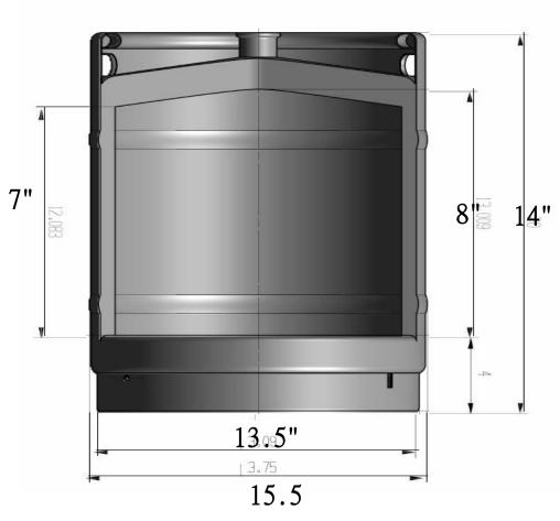
**ENGINEERING SPECIFICATION:** 304 STAINLESS STEELWITH WELDED IN INTREGAL DRAIN 1-1/2"; 3/4" FITTING FOR FLUSH VALVE; BRACKETS FOR MOUNTING; **NO SHARP EDGES. WT. 19 LBS**
