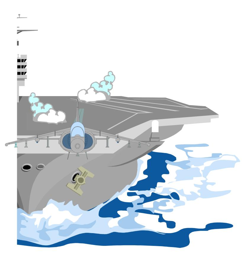
There is a runway atop and a lower deck which becomes a floating hanger. The ship is 17 stories high with four elevators which are used to bring the aircraft up and down from the hanger deck to the flight deck.
