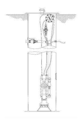
G-Series Gatorgrinder Grinder Pump Station with Wired Level Sensor
