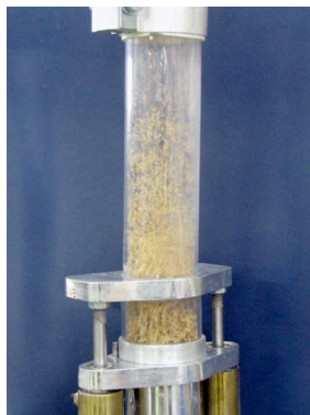
LEFT: Testing for can velocity and terminal velocity are done in a vertical tube
