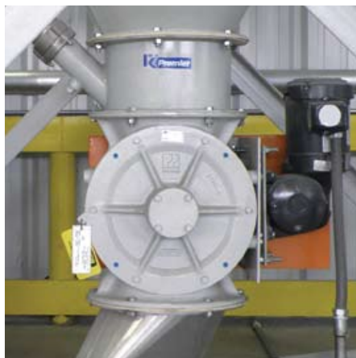
From left: K-Tron Premier Aerolock™ rotary valve in a plastics compounding system; Aerolock™ rotor pockets
