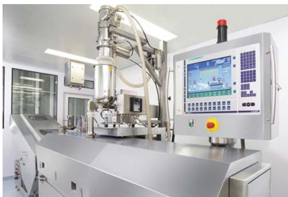
Use of TSEs coupled with accurate LIW feeding and pneumatic refill systems is quickly becoming the manufacturing process of choice when developing pharmaceutical solid dosage forms.
