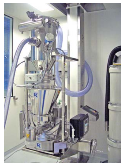
LIW pharmaceutical feeder with integrated vacuum receiver for refill.
