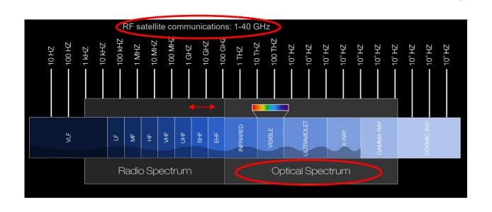
For higher throughput, need to leverage the optical spectrum
