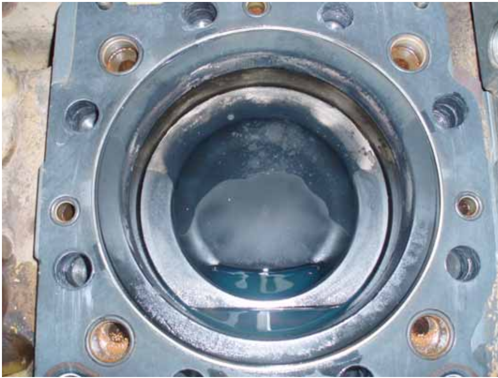
Photo after 51 operating hours using [Private label version of DX1]
