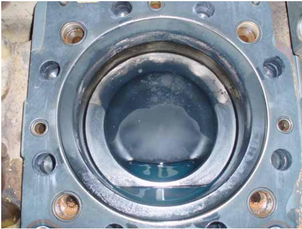
Photo after 51 operating hours using Gamma88
