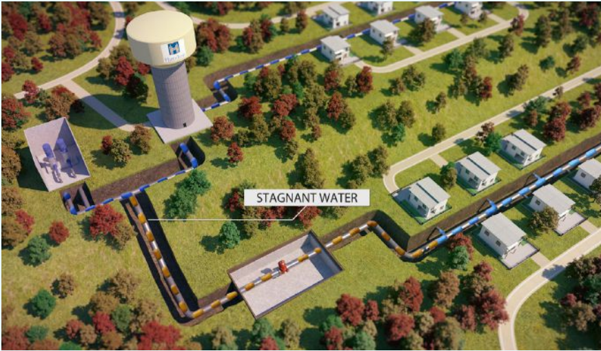
A normally-closed Zone Boundary Valve creates two dead ends, resulting in stagnant water.
