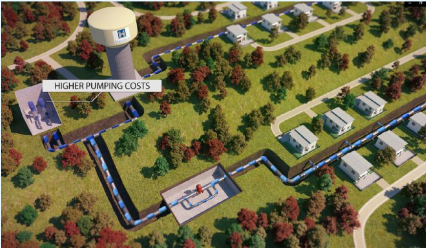
3/4-in. bypass line eliminates stagnant water but (1) increases pumping costs, (2) increases main breaks, (3) instigates in-chamber “mini-breaks.”
