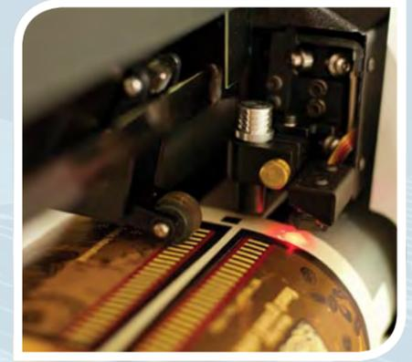
Optical sensors read up to 3 registration marks which ensure the best accuracy in the industry.
