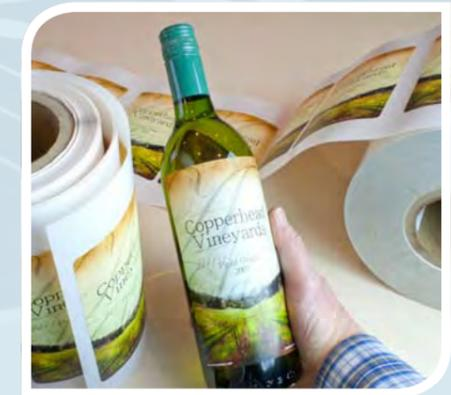
Roll to roll labels, laminated, contour cut with matrix removed and slit into individual rolls - ready for application.
