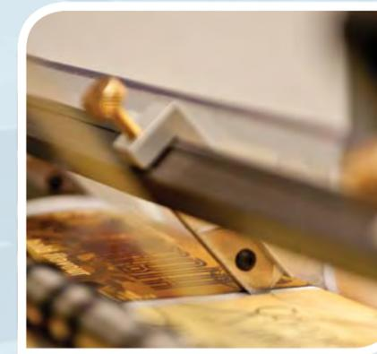
Slitting blades allow for roll slitting, at any width, with up to 5 blades. (3 blades supplied as standard with machine).
