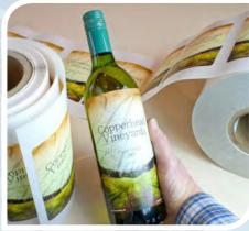
Roll to roll labels, laminated, contour cut with matrix removed and slit into individual rolls ready for application.
