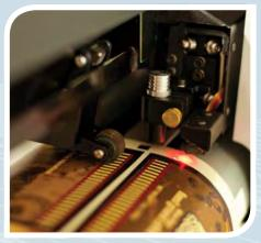
Optical sensors read up to 3 registration marks which ensure the best accuracy in the industry.
