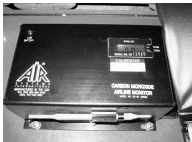
Carbon monoxide monitor
