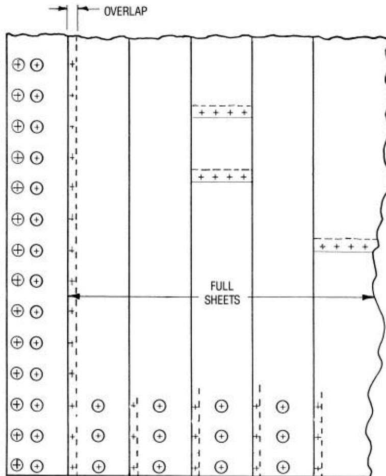
ENDS OF SHEETS ARE LAPPED  $4\frac{1}{2}$ " TO ALLOW FOR FASTENING AND WELDING. FASTENERS ARE INSTALLED ON 12" CENTERS, FLUSH WITH BOTTOM EDGE. ALTERNATE PERIMETER FASTENING WHERE HALF-STRIPS ARE NOT USED IS SHOWN. TOP FASTENERS WITH FASTENER COVERS PLACED IN CENTER OF STRIPS AS INDICATED. FASTENERS GENERALLY PLACED ON 12" CENTERS FOR THE FIRST SIX FEET OF STRIPS FROM EDGE. (SHOWN AS ⊕)
