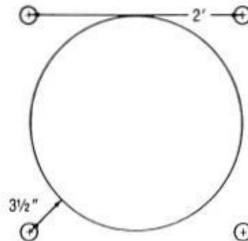
1. FOUR FASTENERS SPACED IN 2' CENTERS, 20" DIAMETER UP TO 30" DIAMETER.
