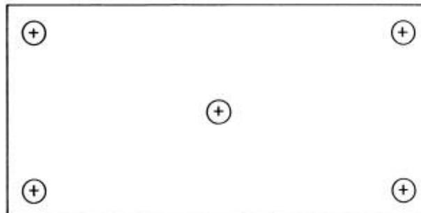
NOTE: THESE FASTENING PATTERNS ARE MINIMUM RECOMMENDATIONS. FACTORY MUTUAL I-60 AND I-90 APPROVED PATTERNS MAY VARY, ACCORDING TO THE INSULATION INVOLVED, AND SHOULD TAKE PRECEDENCE OVER THESE MINIMUMS FOR FM-APPROVED INSTALLATIONS. CONSULT INSULATION MANUFACTURER FOR DETAILS. USE 3" FASTENER PLATES FOR INSULATION FASTENING.
