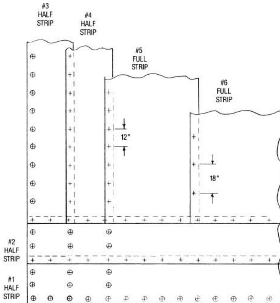
TOP FASTENERS WITH REINFORCED FLEXION FASTENER COVERS (SHOW AS ⊕)
