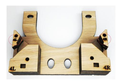
Step 9: Lay the final top pieces on top. (Laser scorched side down.)
