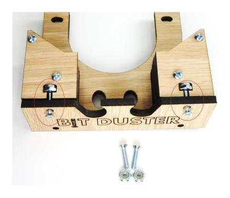
Step 17: Flip the Bit Duster over and screw in the bottom 2 Short Machine screws and 2 Lock nuts. Fully tighten bottom and top screws now.
