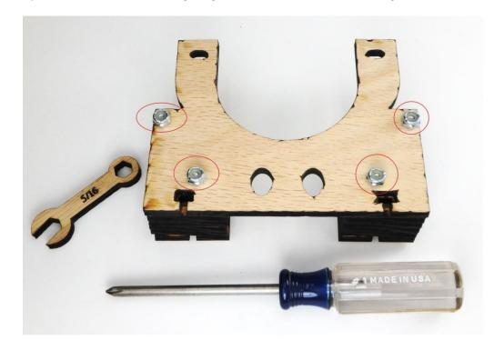
Step 13: Use a Phillips screw driver and the wooden wrench provided to tighten the nuts. Either wrench end will work.
