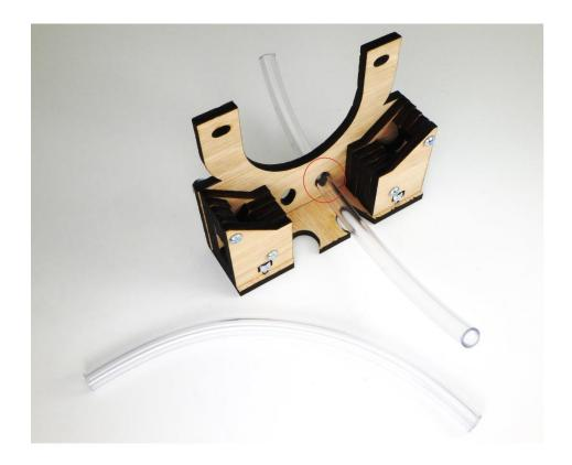
Step 20: Bend the hose around the front and into the side hole.
