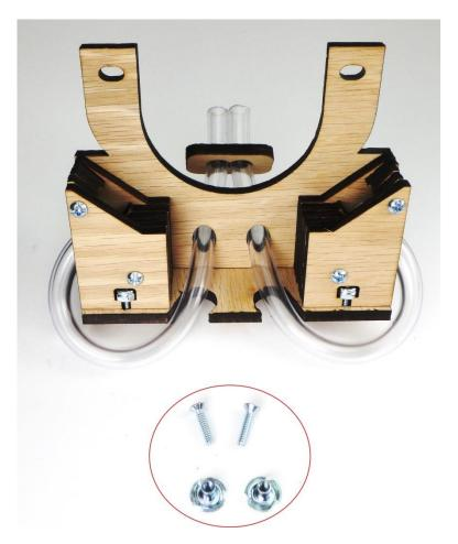
Step 26: Mount the Bit Duster underneath the front of the E3\E4 CNC. Aligning the CNC and Bit Duster holes.
