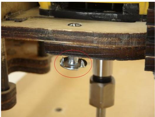
Step 29: Use a screw driver to tighten the Tee Nut until tight.
