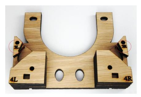
Step 8: Lay Short **4L** on the **L** side and Short **4R** on **R** Side.
