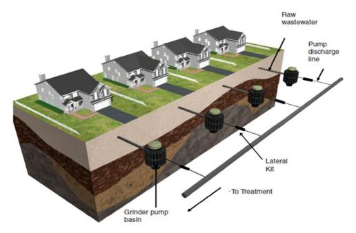
Figure 6 provides an overview of a low-pressure sewer system.
