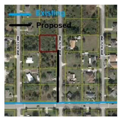
Generally, in Basswood area, the OUA installs approximately 600 LF of 6-Inch piping, a fire hydrant and then 500 LF of 2-inch piping to complete the road. However, there is only one existing house on this road past the subject property. It would not be cost effective to extend the piping for one house.
