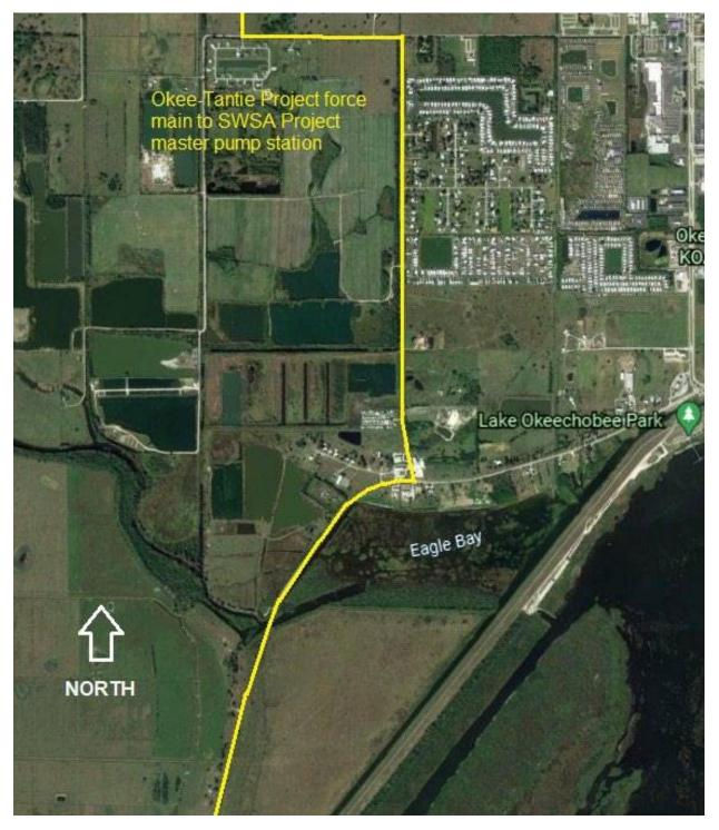
Figure 4. Okee-Tantie to SWSA master pump station (con't)
