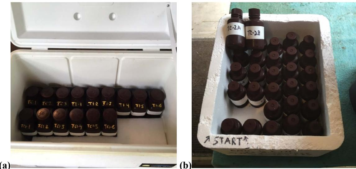
**Figure 21:** Sample collection bottles and coolers. (a-left) 500 mL bottles, water for all analyses except sucralose. (b-right) 60 mL bottles for sucralose analyses.
