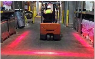
The overhead crane safety warning light system and vehicle safety light could ensure the safety of pedestrians by projecting safety lines on the floor. Those lines (displayed in a chosen colour) inform the people nearby about the moving load and indicate that the overhead crane and vehicle are in operation. It could also help the crane operator position the crane precisely.
