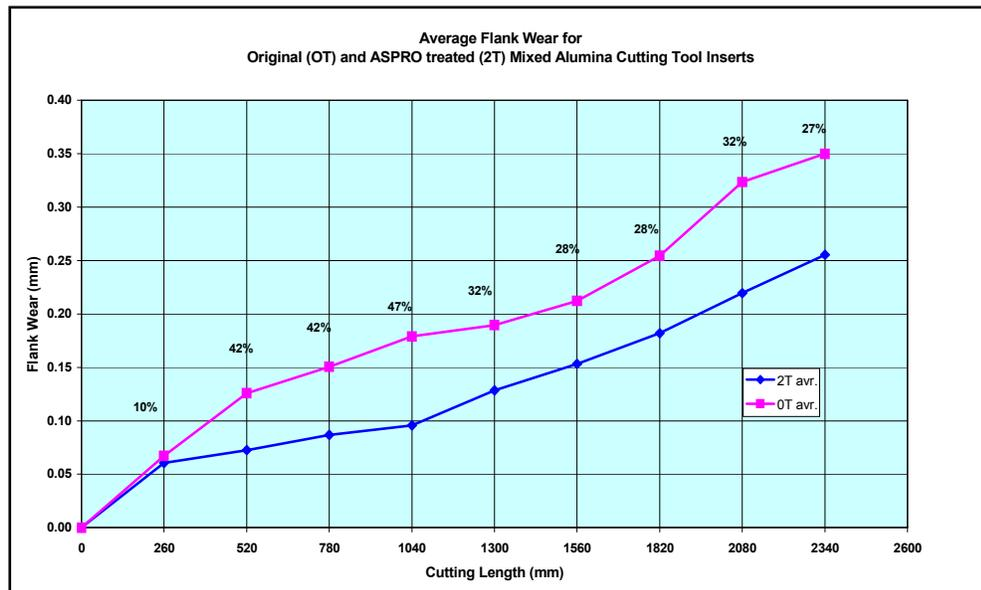
Remarks: Percentages indicate overall improvement in Flank Wear of ASPRO™ treated inserts vs. original inserts at corresponding cutting length.
