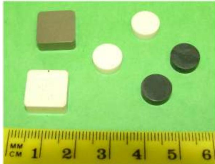
Fig. 1. The ceramic cutting tool inserts.
