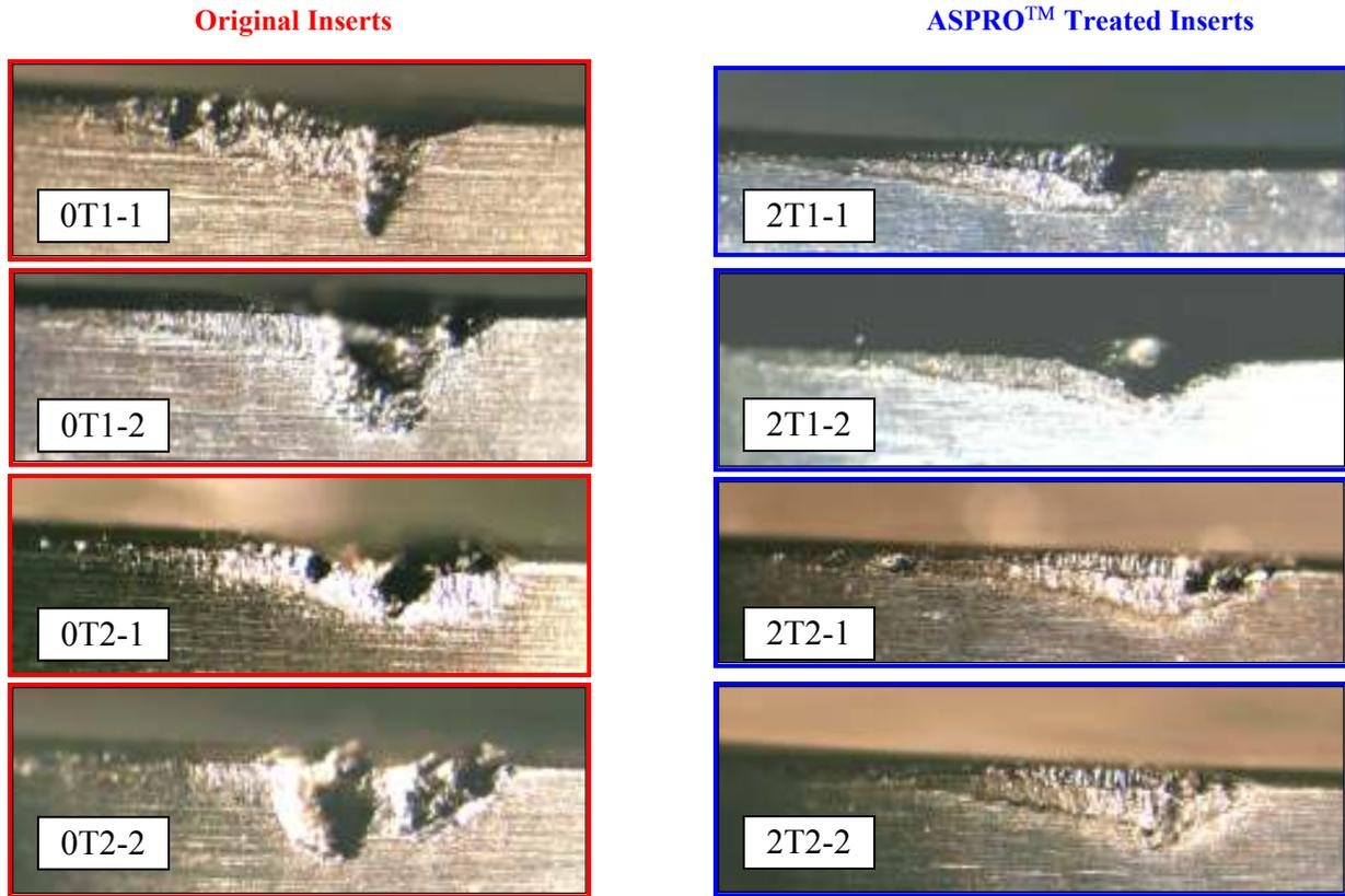
Remarks: Original inserts are marked as 0T1-1, 0T1-2, 0T2-1, 0T2-2 and ASPRO™ treated inserts are 2T1-1, 2T1-2, 2T2-1, 2T2-2.
