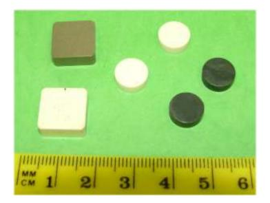
Fig. 1. The ceramic cutting tool inserts.
