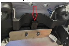
Place the front spacer between the fender and the factory cross bar and attach with the supplied bolts.
