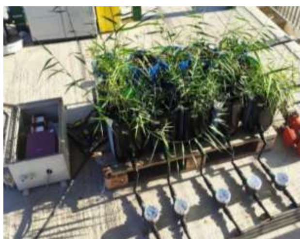
Figure 2 – View of the VF-CW experimental setup.
