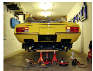
Reassembled rear suspension back on car
