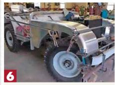
**PANELS GOING ON** Hand-made and -fitted in the traditional way.
