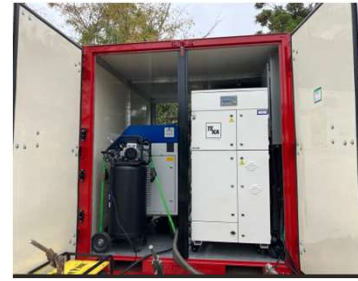
Equipment Container w/Laser System, Induction Unit, Fume Extractor
