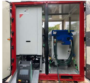
Equipment Container w/Laser System, Induction Unit, Fume Extractor
