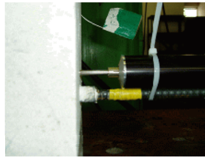
Figure 4. Measurement of slip of each reinforcement
