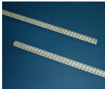
Figure 1. Newly-developed GFRP rebar.
