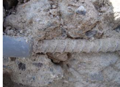
Figure 9. Detail view of bonded and unbonded section
