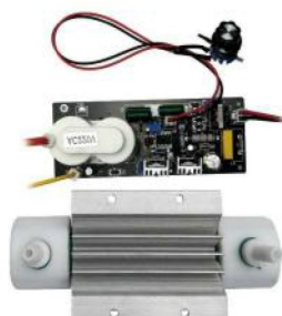
■ 5G double cooling ozone tube + 60W un-adjustable power supply
