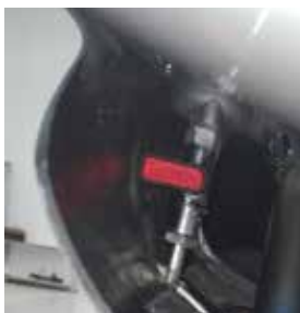
Fuel/water drain outlet
