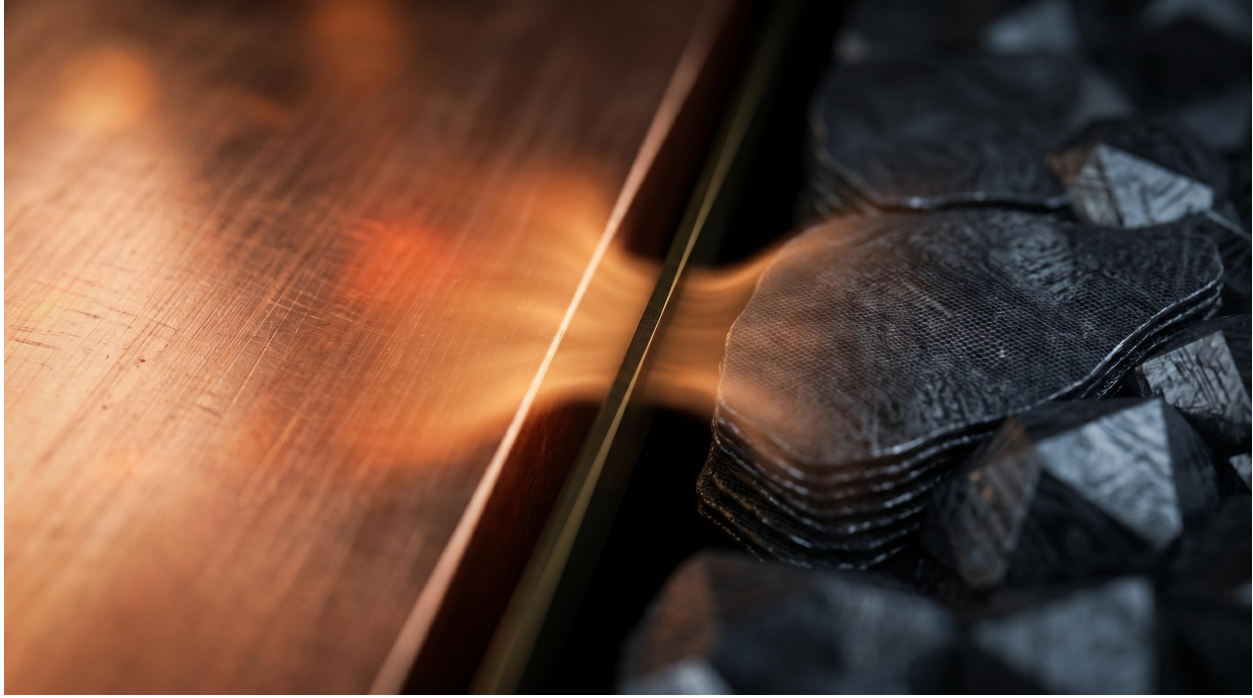
Figure 2: The carbide bridge, in concept. Copper (left) and graphitic carbon (right, rendered as stacked graphene platelets) cannot bond directly—the bare junction is non-wetting, and heat stalls there. The luminous interlayer spanning the gap is the few-nanometer carbide bridge: the thin, continuous phase that couples the two materials and lets heat cross. It is the small structure on which the entire composite’s performance turns, and the locus of the defensible engineering described in Section 4.
