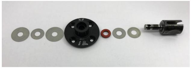
This has been the best starting point with the gearing. If you add shims on the outdrive side the internal mesh will loosen slightly. If you add shims behind the side gears the mesh will tighten. Shim to the best feel.
