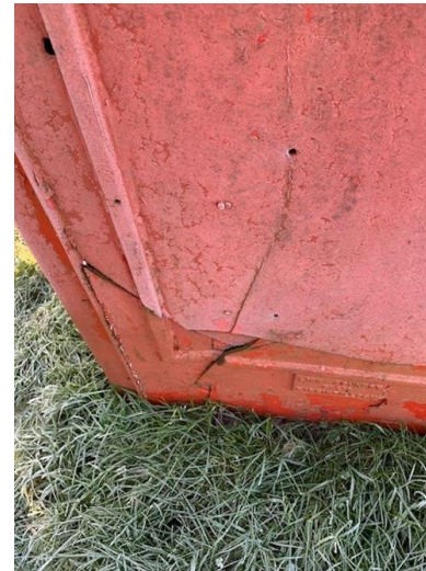
Damage to rear casting.
