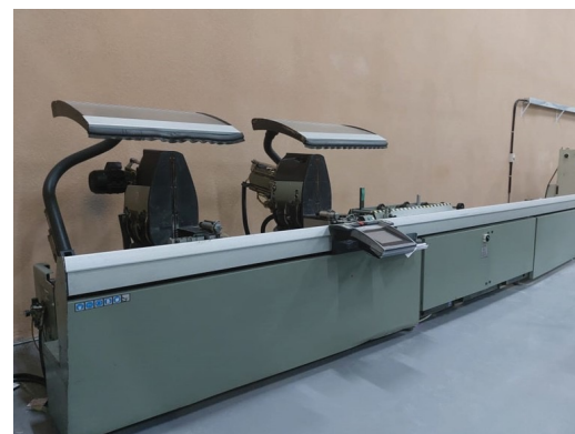
Cnc Double Head Cutting Machine Emmegi Precision Ts 2 Function: 2 Axis Straight And Degree Cutting
