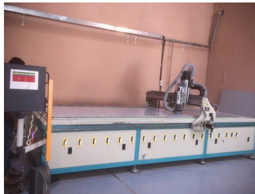
Cnc Cladding Machine Yilmaz Cpm 4150 Function: 3 Axis Composite Panel Processing
