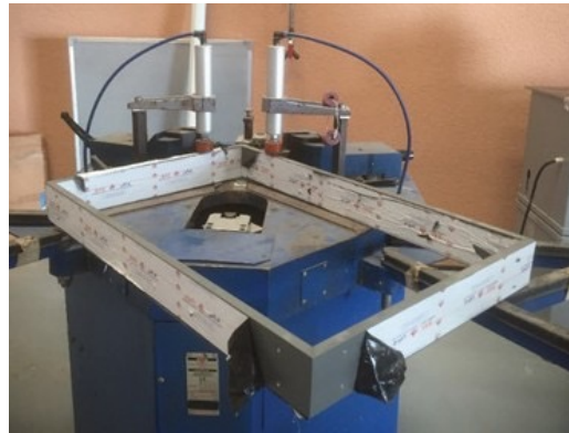
Corner Crimping Machine Atla Coop & Form Industries Function: All Types Of Corner Crimping
