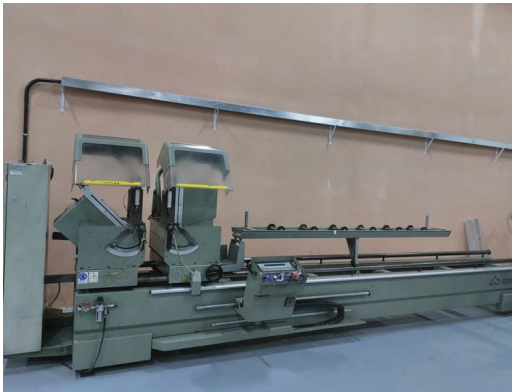
Manual Cutting Machine Emmegi- Classic Magic 500 Function: Straight And Degree Cutting
