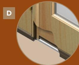
**D** Center mull is integrated into the sill design for higher structural performance
