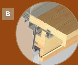
One-piece, full 4<sup>9</sup>/<sub>16</sub>" head and side jambs with inside stop blind nailed to reduce the number of visible nail holes
