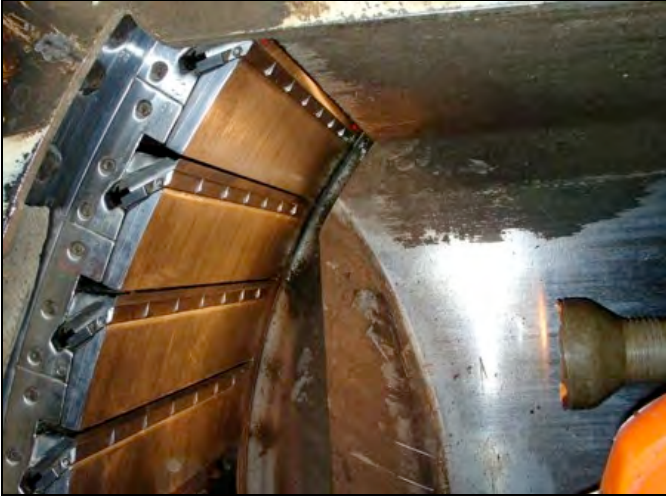
Figure 4.2: Knives in Rotating Strander Drum (With permission of IDAC Logic©)
