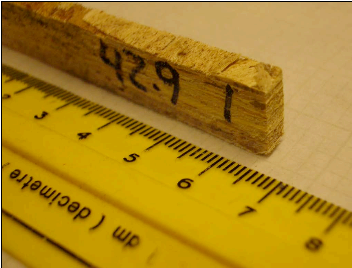
Photograph 5.4: Full Thickness Sorption Slice Specimen, 42.9 lbs/ft 3 Unit Weight (689 kg/m 3 Density).
