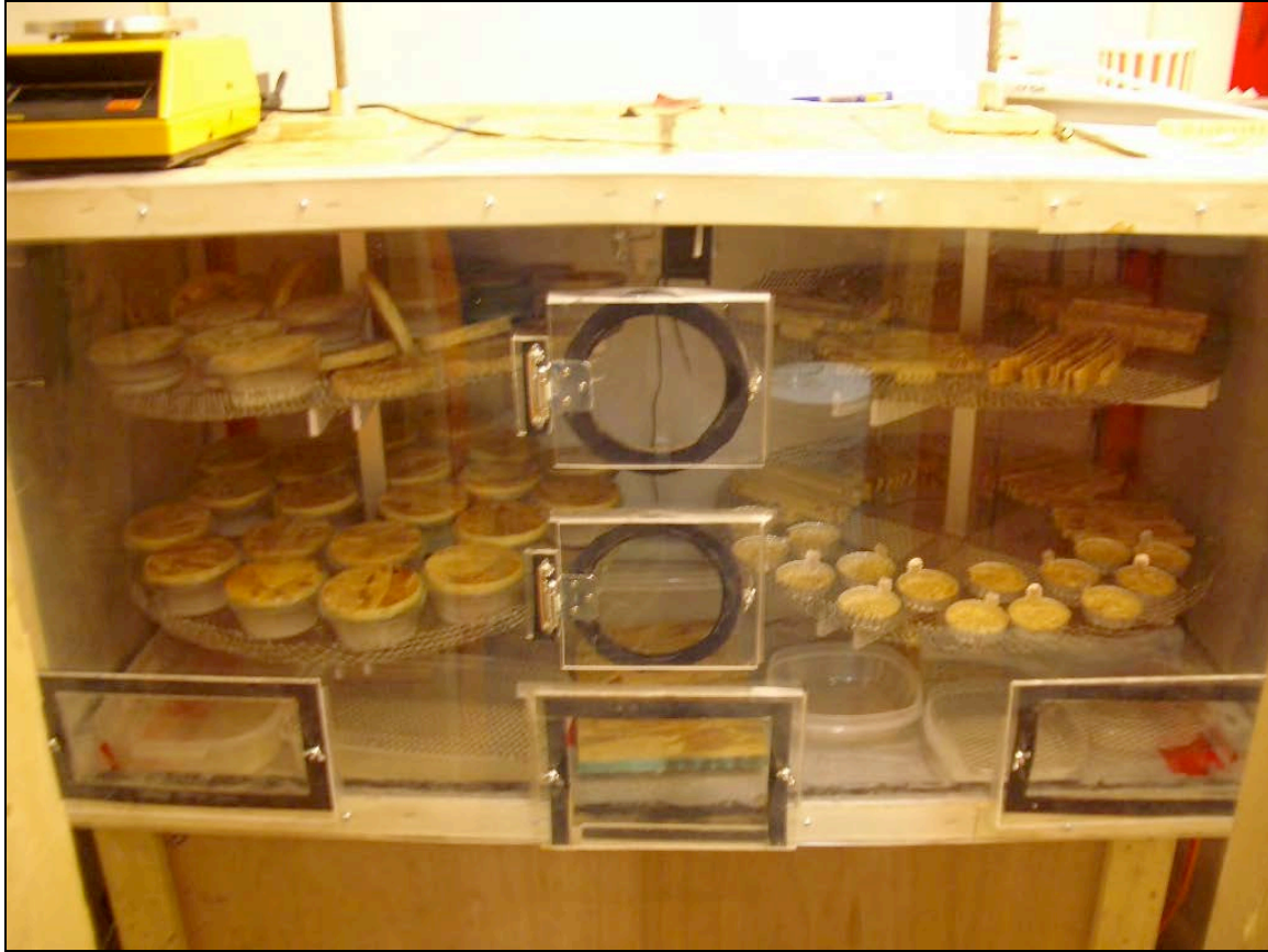
Photograph 5.9: Test Chamber, Temperature and Relative Humidity Controlled, Within Guard Room, Inside Temperature-Controlled Climate Simulator, for Both Permeance and Sorption Testing.
