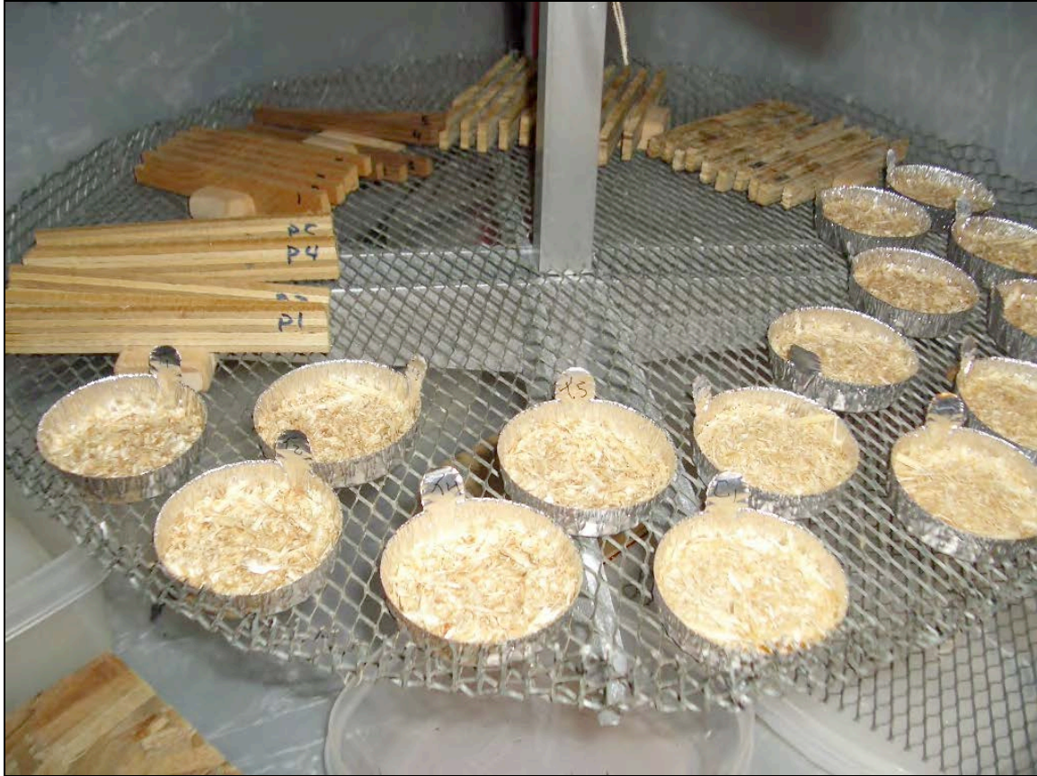
Photograph 5.10: Various Sorption Test Specimens in Controlled Temperature and Relative Humidity Chamber During Testing.
