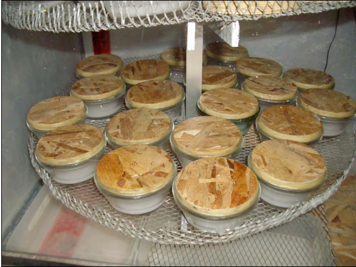
Photograph 5.8: Permeance Cup Test Assemblies in Controlled Temperature and Relative Humidity Chamber.
