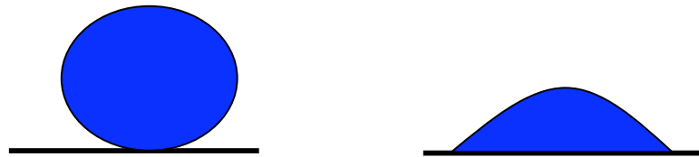
Figure 3.2: Water Drop on a Hydrophobic (left) and Hydrophilic (right) Surface.
