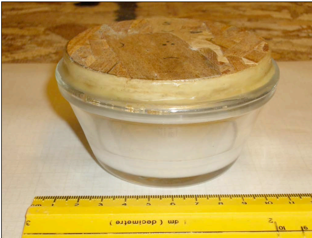
Photograph 5.7: Permeance Test Assembly, Cup with Saturated Salt Solution and Full Thickness OSB Test Specimen Sealed to Cup with Parafin Wax.
