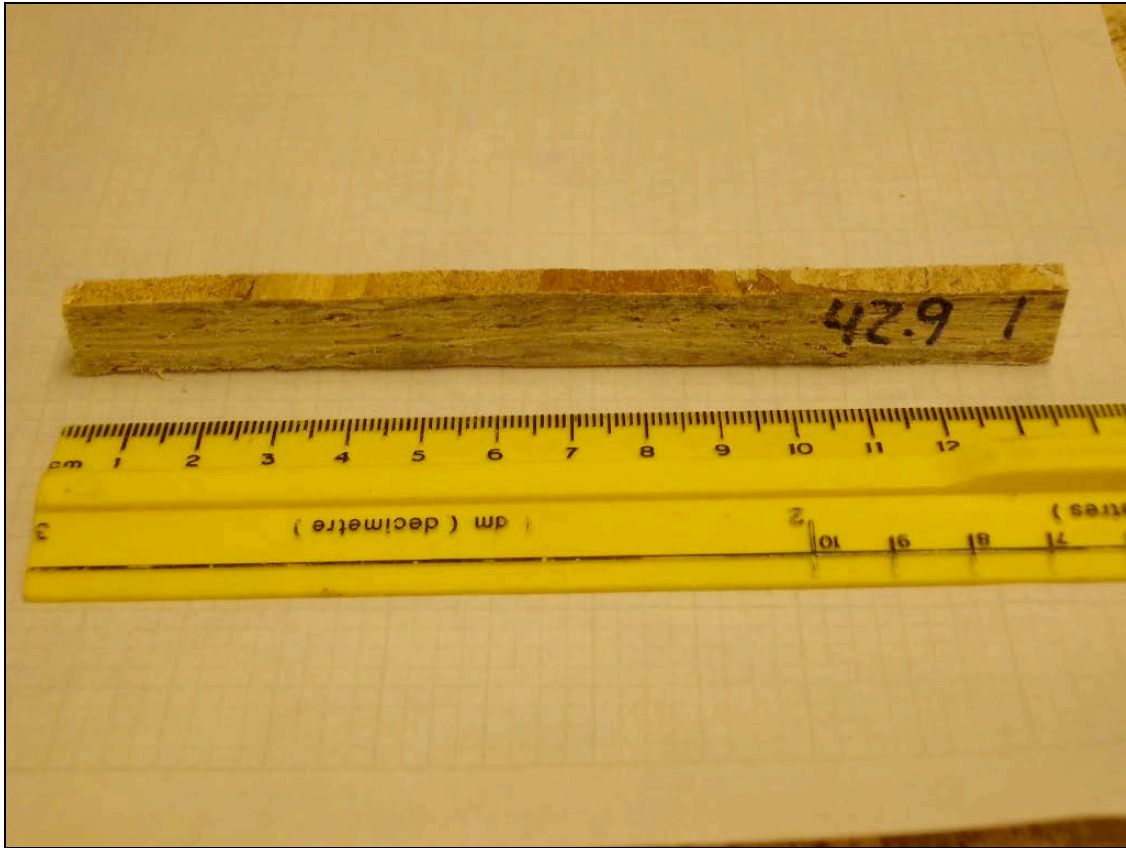
Photograph 5.3: Full Thickness Sorption Slice Specimen, 42.9 lbs/ft 3 Unit Weight (689 kg/m 3 Density) Group.
