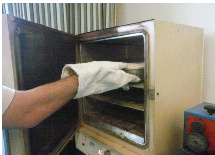
Fig. 2. Oven used to dry waste wood
