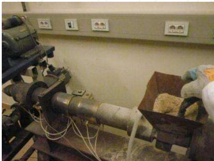
Fig. 3. Feeding the extruder with the mixture
