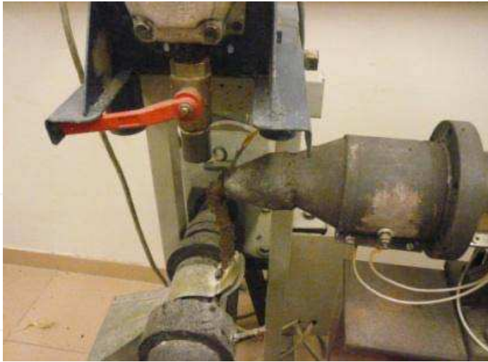
Fig. 4. The hot extrudates coming out of the extruder
