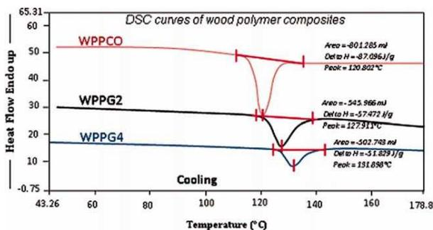
**Figure 4** DSC curves of WPCs with different MAPP contents (the curves were vertically moved for clarity). The compositions of the samples are described in Table I. [Color figure can be viewed in the online issue, which is available at [wileyonlinelibrary.com](http://wileyonlinelibrary.com).]
