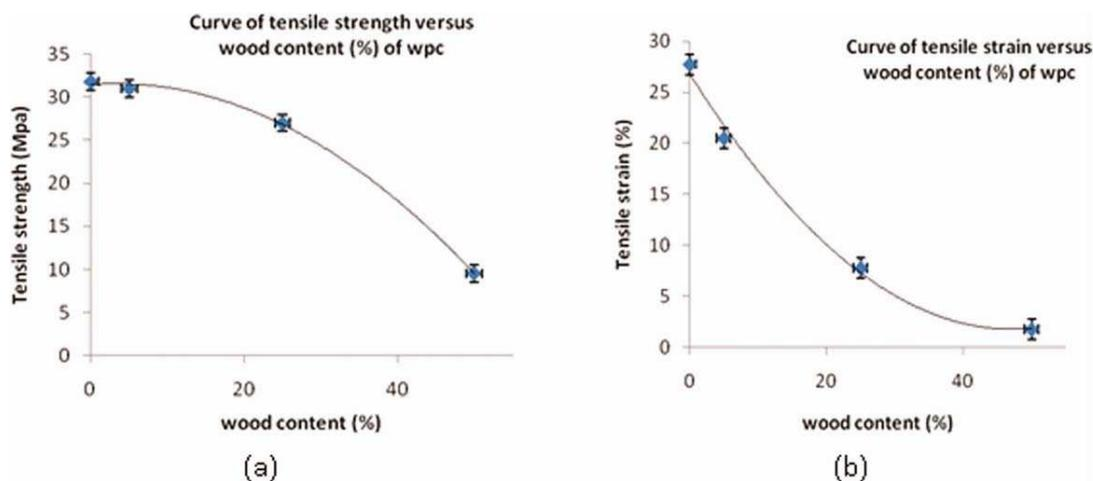
**Figure 6** Effect of the wood flour content on the tensile strength and tensile strain of the WPCs. No coupling agent or clay was used in the composites. [Color figure can be viewed in the online issue, which is available at [wileyonlinelibrary.com](http://wileyonlinelibrary.com).]
