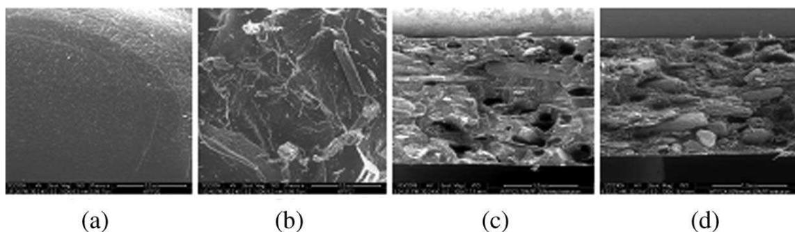
**Figure 1** SEM micrographs of (a) pure PP and composites containing (b) 5, (c) 25, and (d) 50 wt % wood flour.
