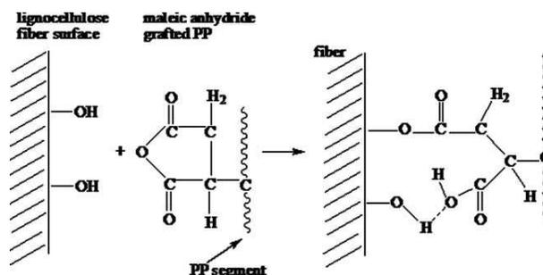
**Figure 3** Reaction mechanisms of MAPP with a hydroxyl group on the surface of the wood flour.
