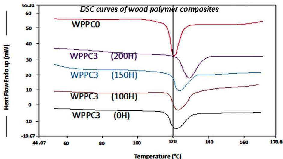
**Figure 5** Thermograms of the pure PP and irradiated WPPC3 (75 wt % PP + 25 wt % wood flour). [Color figure can be viewed in the online issue, which is available at [wileyonlinelibrary.com](http://wileyonlinelibrary.com).]
