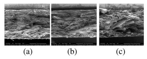
**Figure 2** SEM micrographs for WPCs containing (a) 5 wt % MAPP, (b) 5 wt % clay, and (c) 2.5 wt % MAPP and 2.5 wt % clay. All of the samples contain 50 wt % wood flour.
