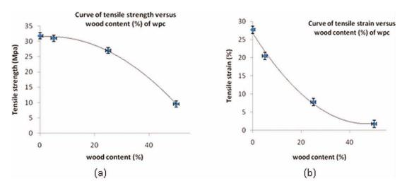
**Figure 6** Effect of the wood flour content on the tensile strength and tensile strain of the WPCs. No coupling agent or clay was used in the composites. [Color figure can be viewed in the online issue, which is available at wileyonlinelibrary. com.]
