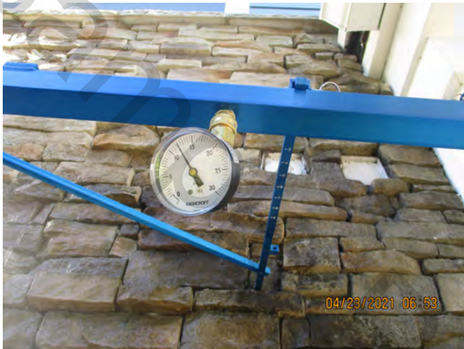
Spray Rack Water Pressure showing 12 PSI
