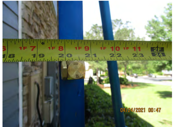
Spray Rack Nozzles 20" from test specimen
