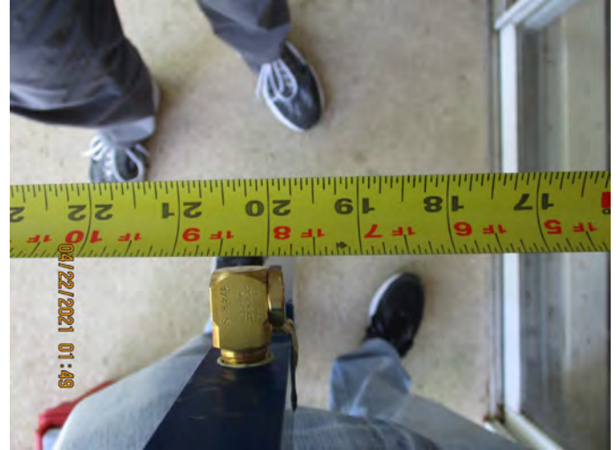
Spray Rack Nozzles 20" from test specimen
