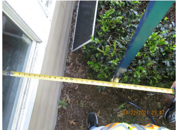
Spray Rack Nozzles 20" from test specimen
