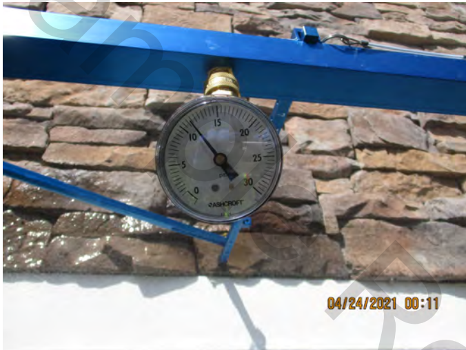
Spray Rack Water Pressure showing 12 PSI
