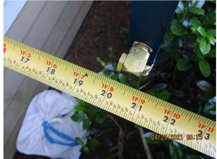
Spray Rack Nozzles 20" from test specimen
