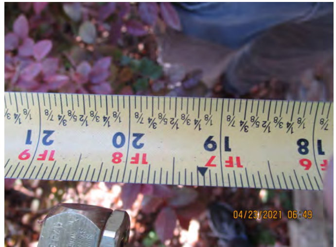
Spray Rack Nozzles 20" from test specimen
