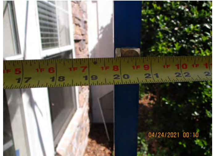
Spray Rack Nozzles 20" from test specimen
