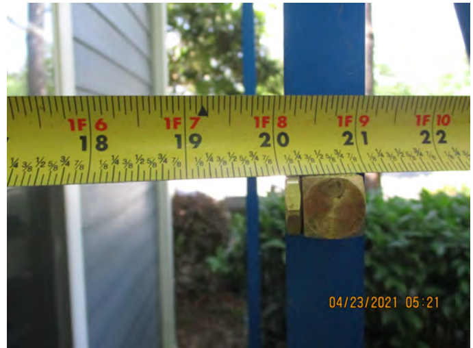
Spray Rack Nozzles 20" from test specimen
