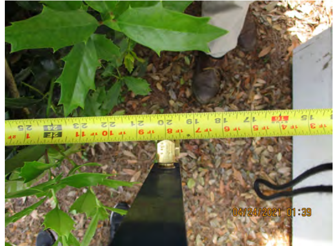
Spray Rack Nozzles 20" from test specimen
