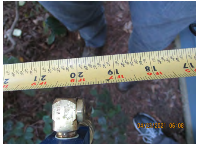
Spray Rack Nozzles 20" from test specimen
