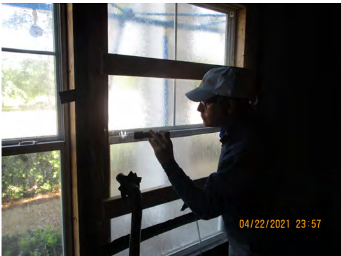
Observing Testing – Looking for water penetration
