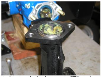
Apply automotive bearing grease to PTO coupler on gearbox, also PTO shaft located at back of transmission (blue housing) and flange mating surface.
