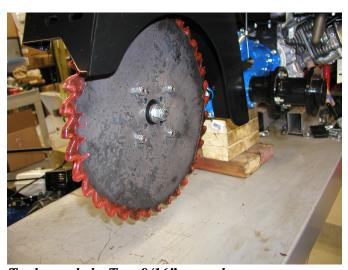
*Tools needed: Two 9/16" wrenches.*Mount blade on blade flange using existing nuts and bolts. Note orientation of blade ó shown as [set up for counter rotation, reverse drive].
