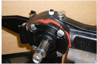
Tools needed: 14mm wrench and 1/4" Hex Key. [Note: Gearbox contains SAE 80/90 or SAE 90 EP (extreme pressure) gear oil]. Do not spill or allow contamination. Secure gearbox in vice with oil drain plug facing up. Using 14mm wrench remove stock oil drain plug and insert threaded pipe plug (use pipe sealant), tighten with ½öhex key. Save stock oil plug for rear mount. Note: Newer gearboxes are sealed so this step can be skipped.
