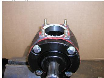
Reuse gasket and use gasket sealer to assure correct seal. Gearboxes are sealed now from the factory.
