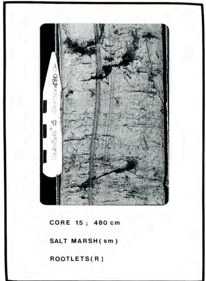
Figure 12. Core 15: salt marsh rootlets in growth position from a massive clay facies at a depth of 4.80 m below the seabed at the mouth of Cumberland Basin. The sample comes from unit G2 and formed approximately 7,000 BP.
